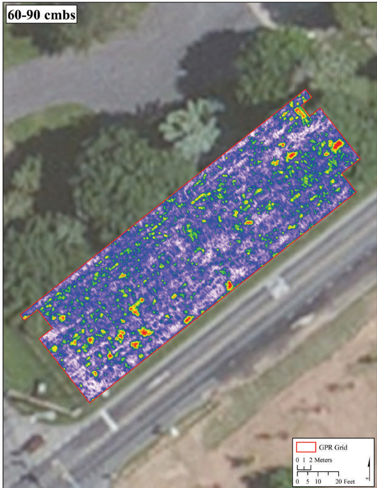
Figure 18. GPR Amplitude Slice Map, 60-90 cmbs
