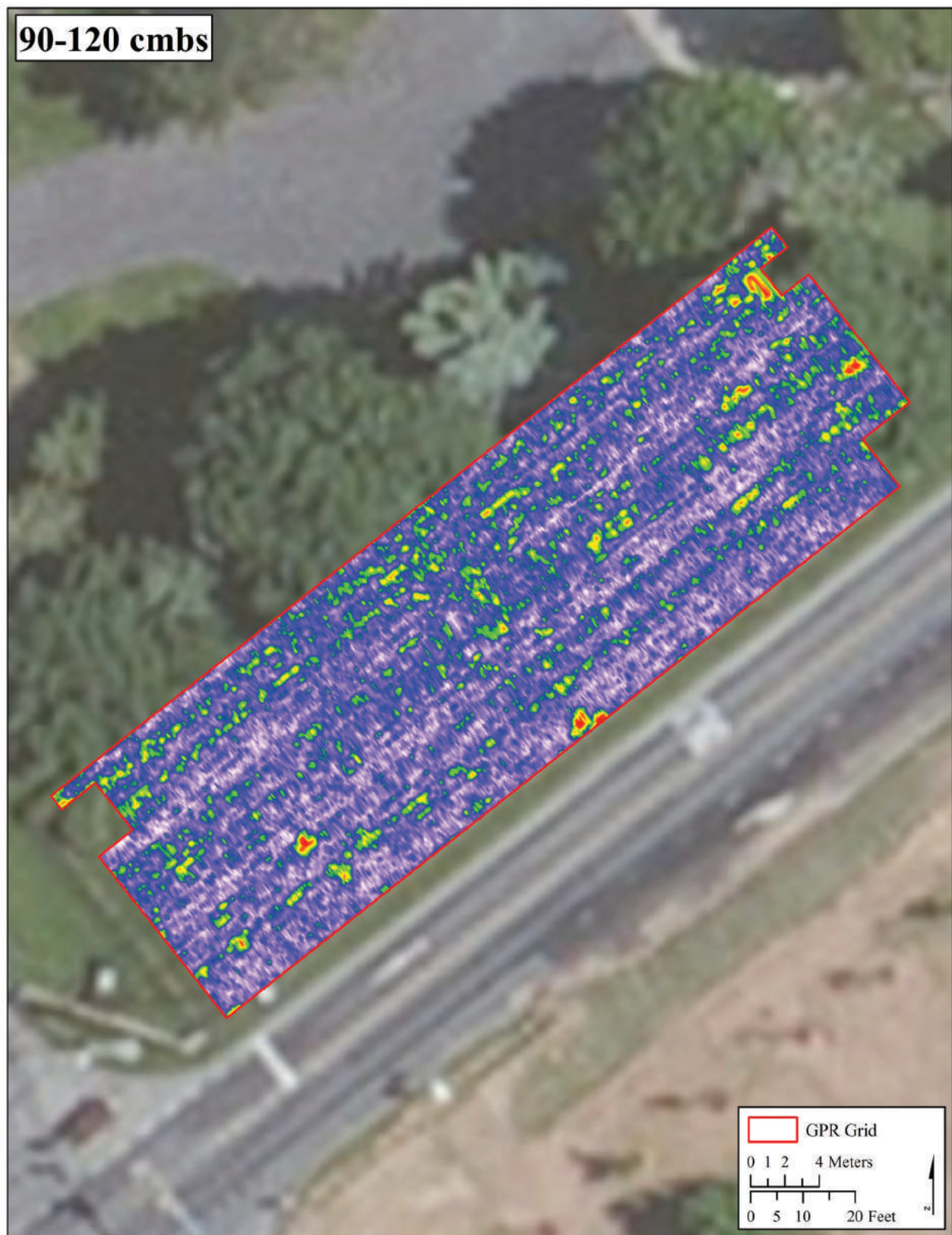
Figure 19. GPR Amplitude Slice Map, 90-120 cmbs
