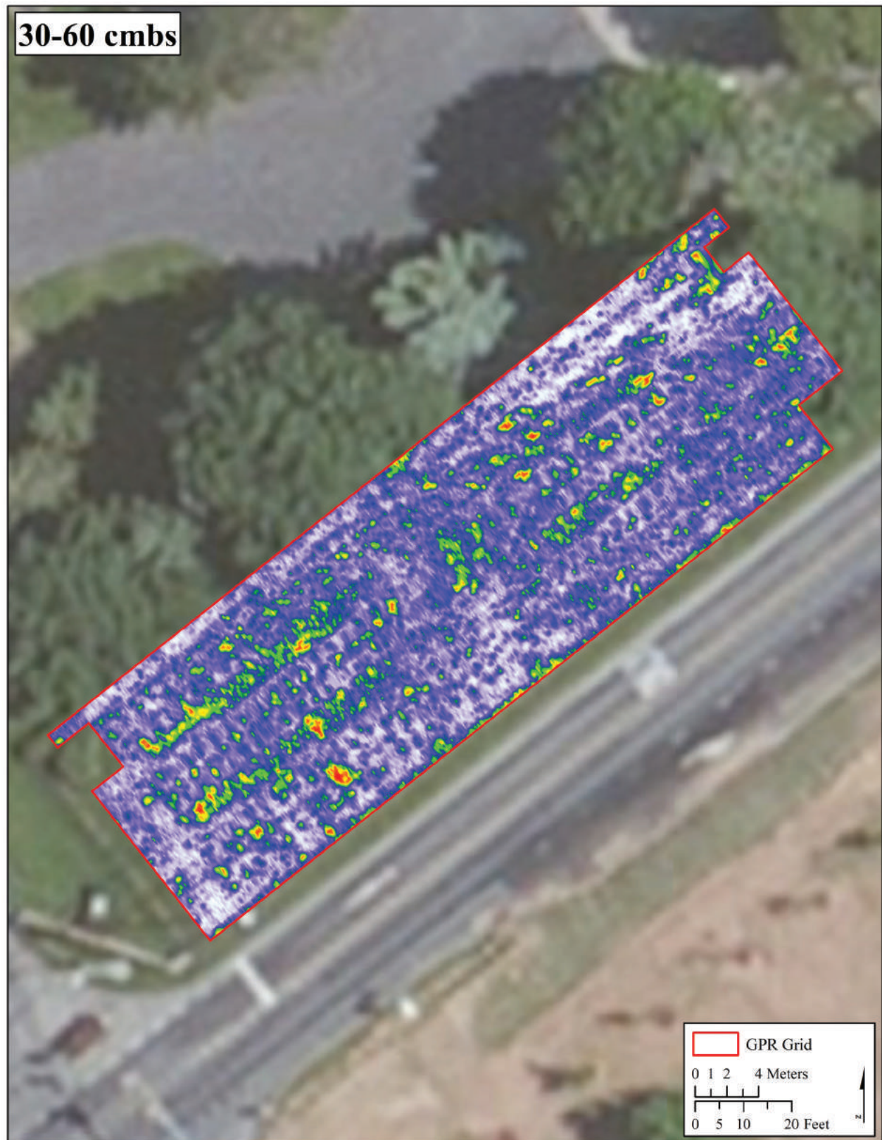
Figure 17. GPR Amplitude Slice Map, 30-60 cmbs
